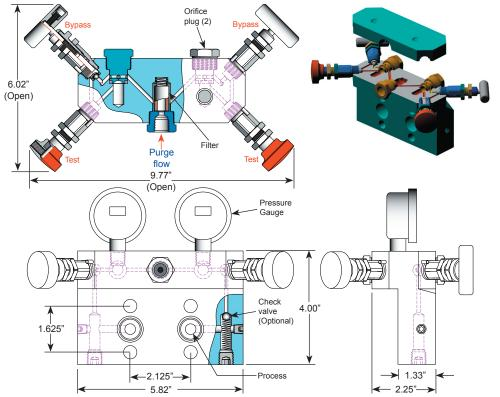
Specifications: Type: P6PM4H Purge Manifold, Globle Pattern Rating: Up to 6000 psi @ 100°F (41370 kPa @ 38°C) Stem: Ball Tip Packing: Teflon™ or Grafoil™ Seat: Integral Handle: Removable Bore Size: 3/8" (Process), 1/8" (Purge) Inlet Connections: 1/2" FNPT x 2 Outlet Connections: 4-bolt Flange Bonnet Lock: Pin or Plate Weight: 11.8 lbs Special Service: O₂ or CL cleaning available\*
