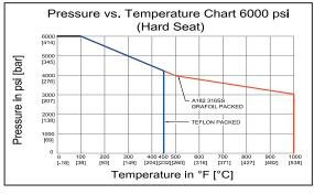
Note: Body material specifications based on ASME B16.34 - 2013. Packing material ratings based on manufacturer's specifications. Approximations only. Parker does not represent these values as finite. They are provided only as representative values.
